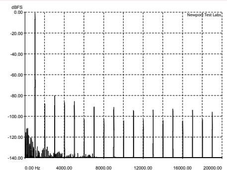
**Graph 3:** Total harmonic distortion (THD) at 1kHz at an output of 350-watts into an 8-ohm non-inductive load, referenced to 0dB. [Redgum Magnificata Power Amplifier]
