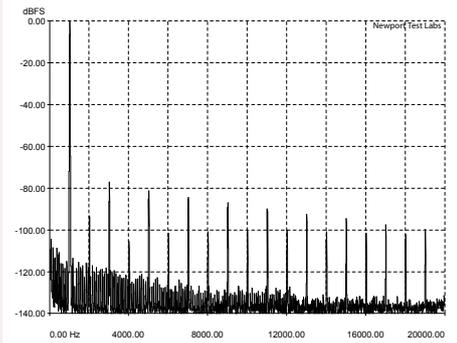
**Graph 1:** Total harmonic distortion (THD) at 1kHz at an output of 1-watt into an 8-ohm non-inductive load, referenced to 0dB. [Redgum Magnificata Power Amplifier]
