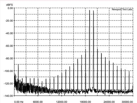
**Graph 5:** Intermodulation distortion (CCIF-IMD) using test signals at 19kHz and 20kHz, at an output of 1-watt into an 8-ohm non-inductive load, ref. to 0dB. [Redgum Magnificata]
