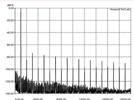
**Graph 2:** Total harmonic distortion (THD) at 1kHz at an output of 1-watt into a 4-ohm non-inductive load, referenced to 0dB. [Redgum Magnificata Power Amplifier]
